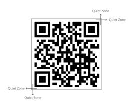
do not interfere with its readability. Providing a clear boundary, the quiet zone improves the accuracy of QR code detection and scanning.
