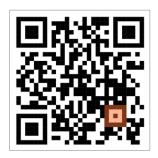
Multiple alignment patterns are placed evenly across the QR code, allowing for accurate reading by correcting both linear and nonlinear distortions.
